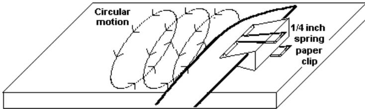
A 1/4 inch spring paper clip attached to the blade back will work as an angle guide.
